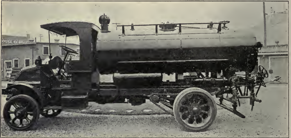
A KINNEY ROAD-OILER MOUNTED ON A KELLY-SPRINGFIELD TRUCK OPERATED BY MARION COUNTY, OHIO, IN MAINTAINING ITS ROADS
